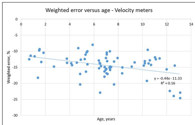
**Figure 6.** Weighted error versus age – velocity meters
