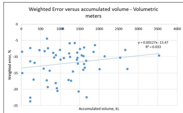
**Figure 9.** Weighted error versus accumulated volume – volumetric meters
