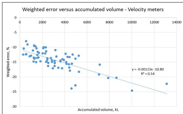
**Figure 8.** Weighted error versus accumulated volume – velocity meters
