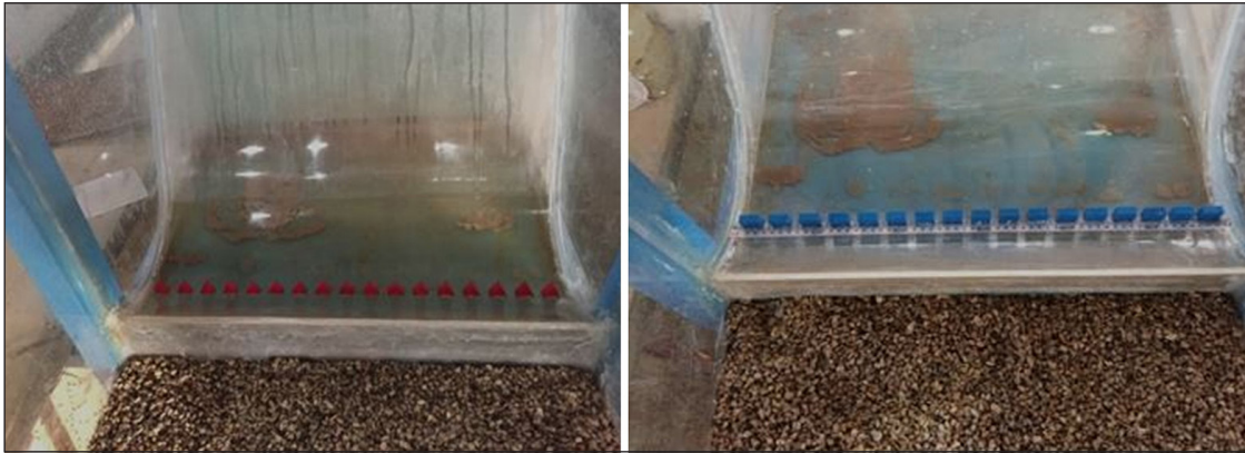
Figure 5. Flip bucket with rectangular and triangular slots in a continuous configuration according to USBR
