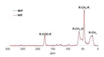
**Figure 3**Solid-state 13C CP/MAS NMR spectra of the MIP and NIP
