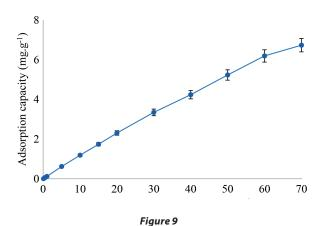
Effect of initial concentration of ketoprofen on the extraction efficiency of ketoprofen by MIP sorbent. Experimental conditions: 10 mL water, sample pH 5, contact time of 45 min, and polymer mass of 8 mg (n = 3).
