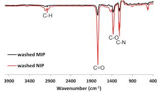
**Figure 4**FTIR spectra of the synthesized MIP and NIP
