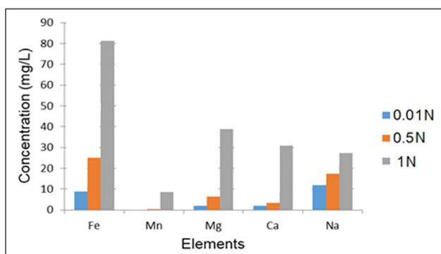
Figure 6. Concentrations of Fe, Mn, Mg, Ca and Na eluted from the resin using different concentrations of sulphuric acid
