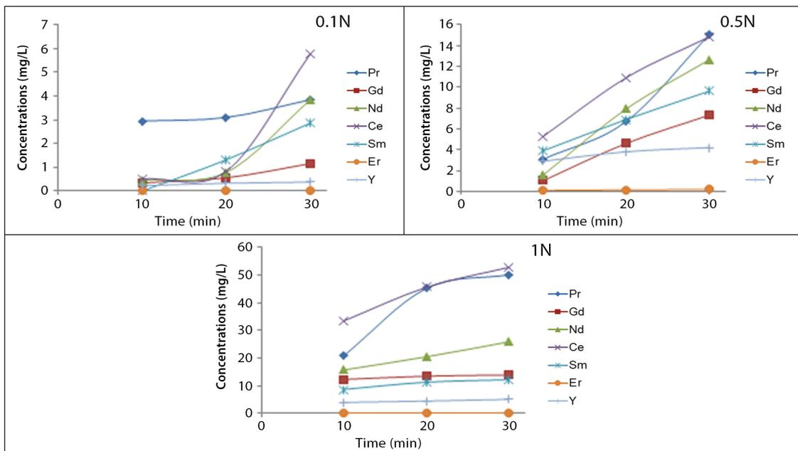
Figure 5. Elution of REEs from sorbed resin with solution of sulphuric acid (0.1, 0.5 and 1 N) for 10, 20 and 30 min
