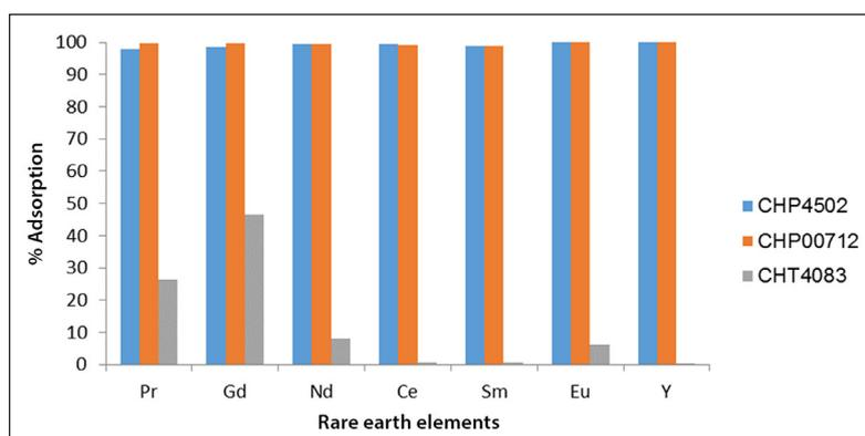
Figure 2. Removal efficiencies (%) for REEs by resins (at pH = 2.37, S/L = 2/5, contact time = 60 min, speed of mixing, = 500 r/min)
