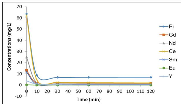
Figure 4. Effect of time on the removal of REEs with CHP00712 resin
