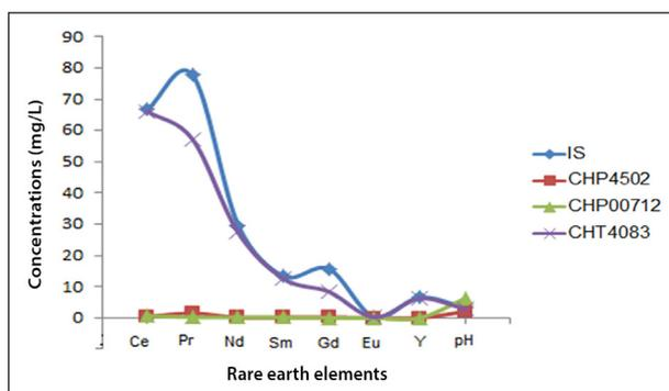
Figure 1. Sorption of REEs on different resins (IS = initial sample)
