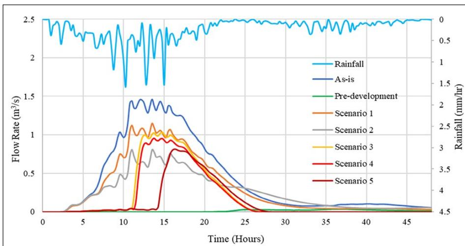
**Figure 32.** Outfall flow rates during a typical storm event (18–21 April 2010)
