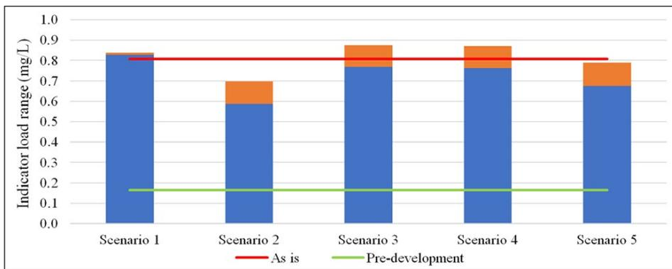
**Figure 30.** TIN model outflow concentrations; eutrophic range of 2.5–10 mg/L; orange bars represent the concentration range due to high and low treatment potentials
