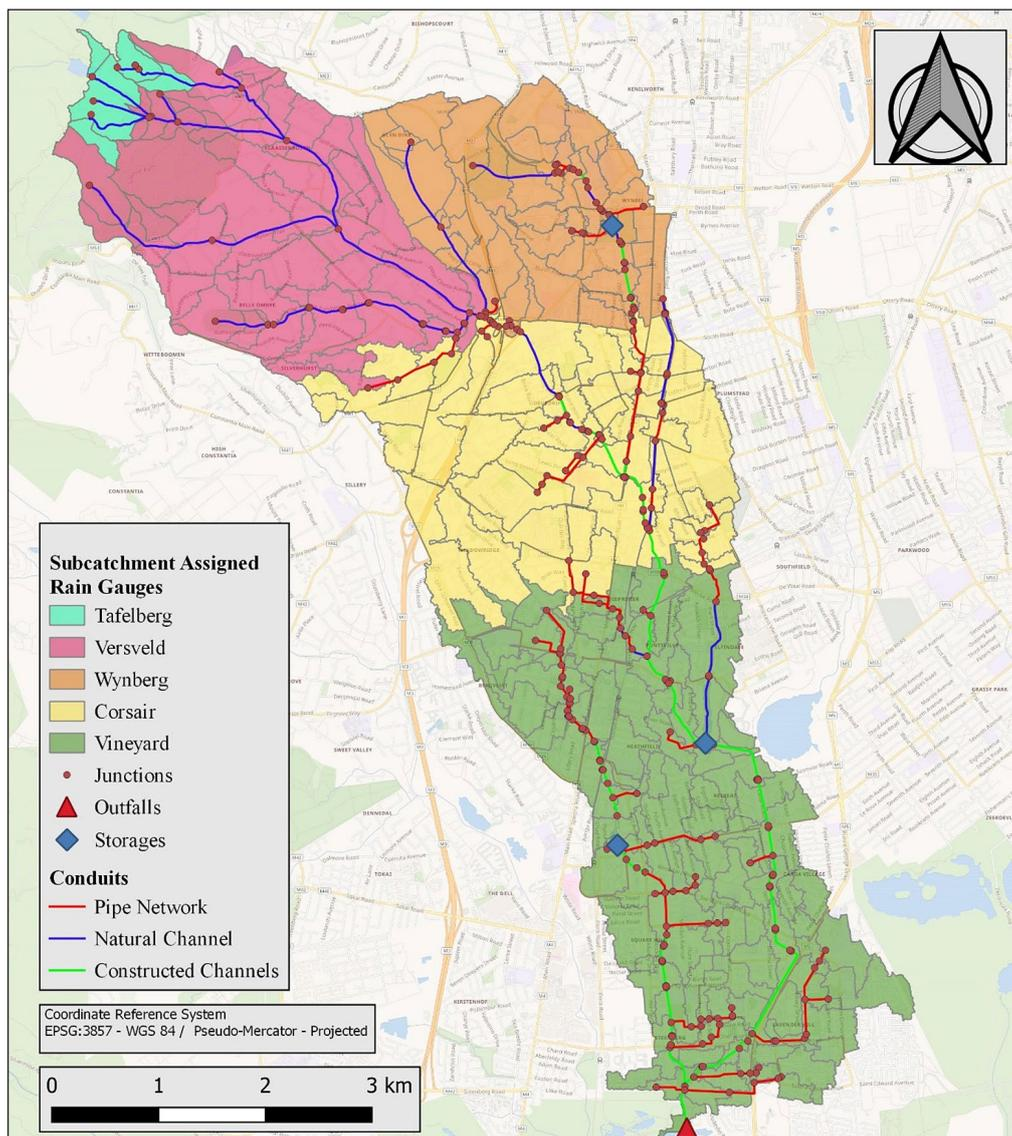
**Figure 3.** Model network showing rain gauge sub-catchments, conduits, storages, and outfall – adapted from Wikimedia Maps (Wikimedia, 2021)
