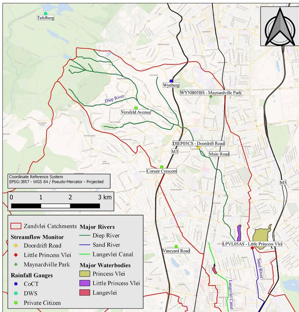
Figure 5. Streamflow monitors and rainfall gauges – adapted from Wikimedia Maps (Wikimedia, 2021)
