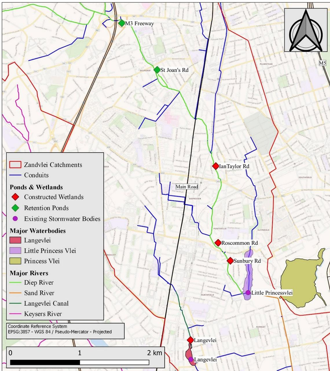
**Figure 19.** Existing ponds and wetlands reincorporated into the drainage system
