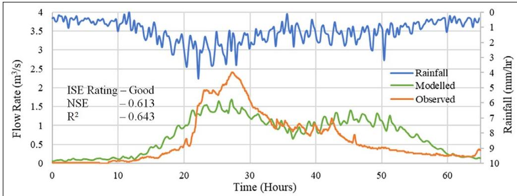
Figure 6. Modelled and observed hydrographs of a typical storm event (27–30 August 2013)
