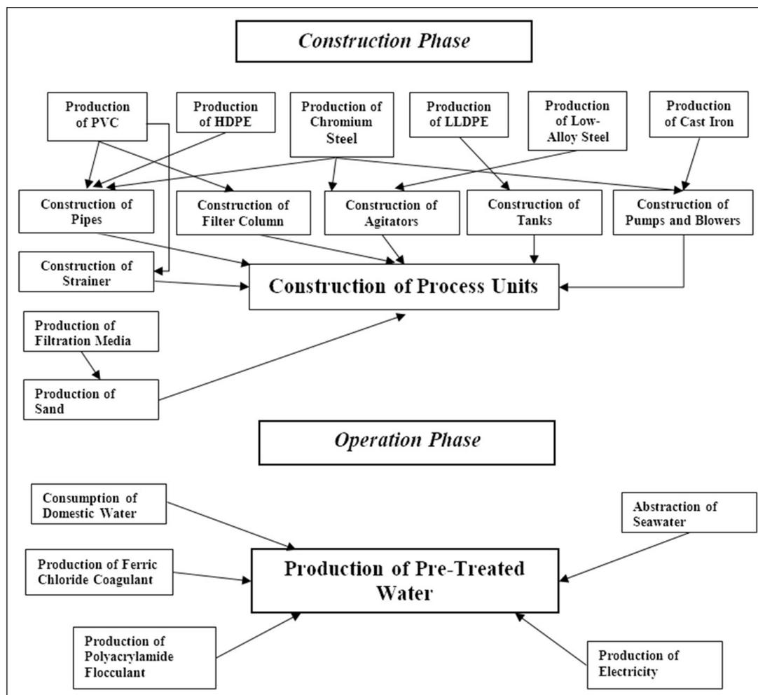
Figure 3. Processes included for System 1 (scope of the LCA inventory for System 1)
