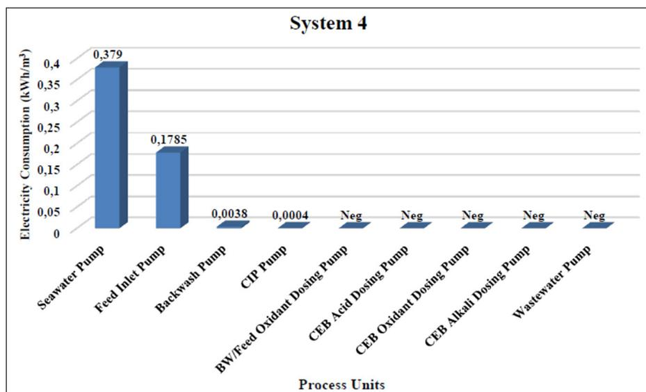
**Figure 12.** Electricity used by process units in System 4
