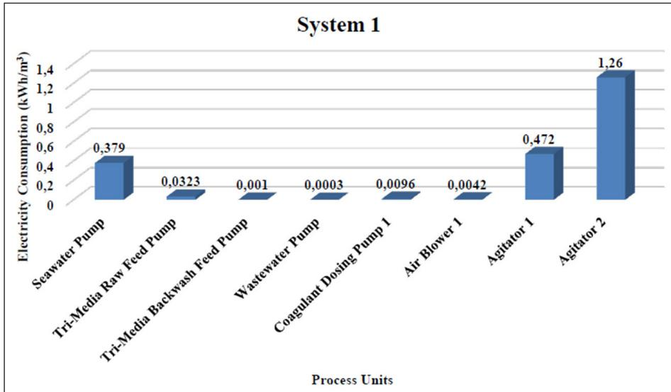
Figure 9. Electricity used by process units in System 1
