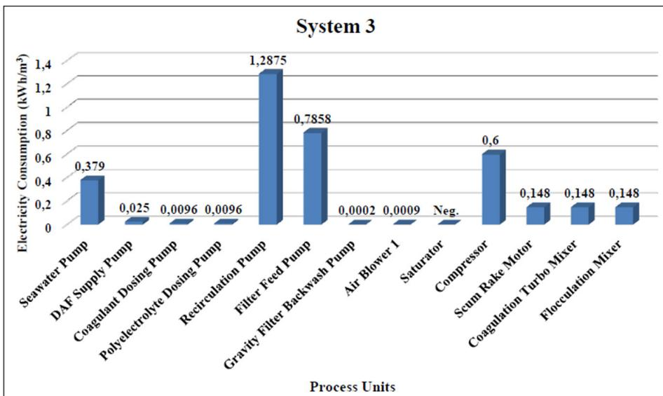
Figure 11. Electricity used by process units in System 3
