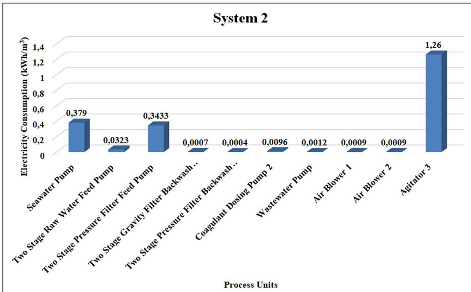
Figure 10. Electricity used by process units in System 2
