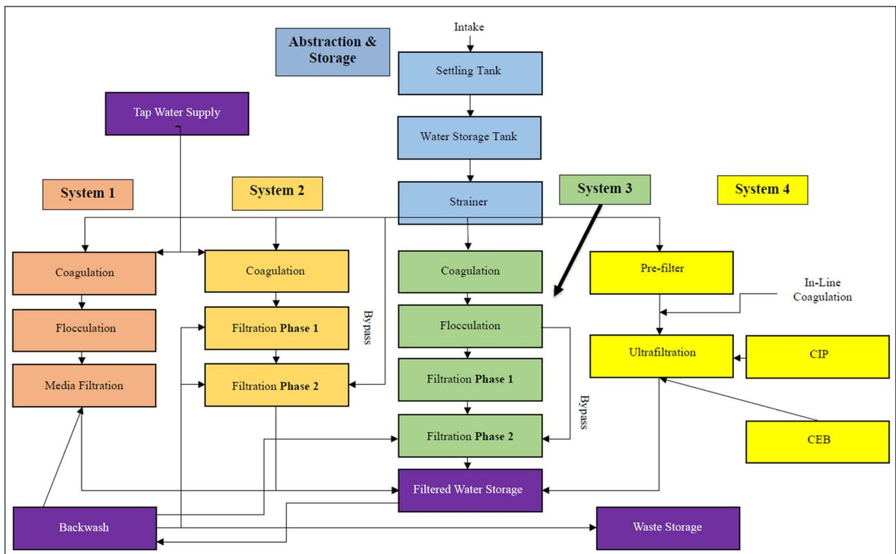
Figure 1. Simplified pre-treatment pilot plant process diagram
