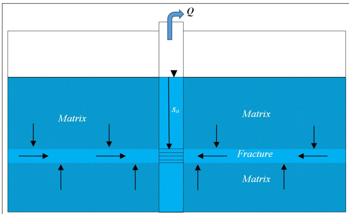
Figure 1. Schematic diagram showing the available drawdown ( $s_a$ ) above the fracture/main water strike
