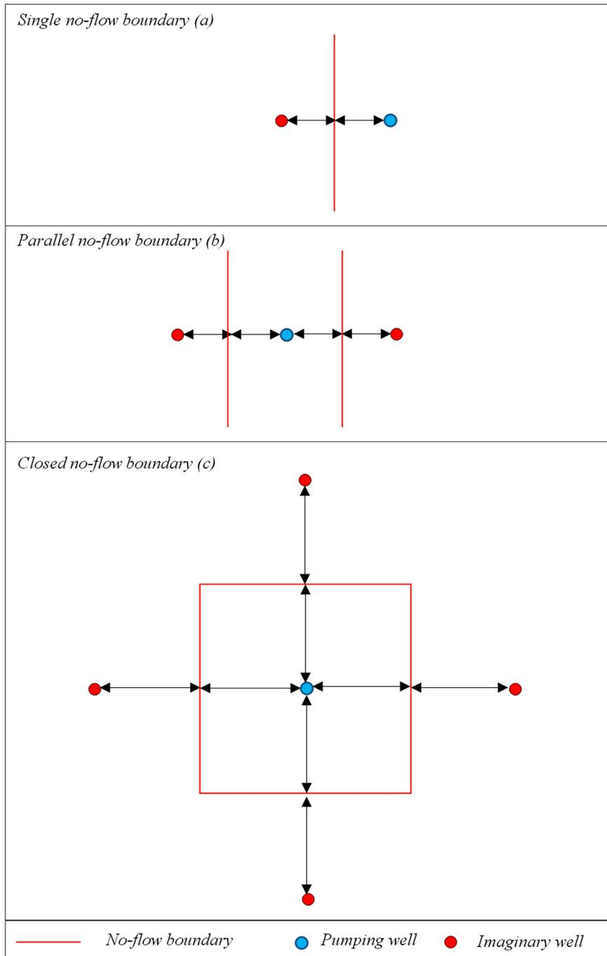
**Figure 2.** Schematic showing the representation of no-flow boundaries using imaginary wells; distance between the wells and boundaries is equal
