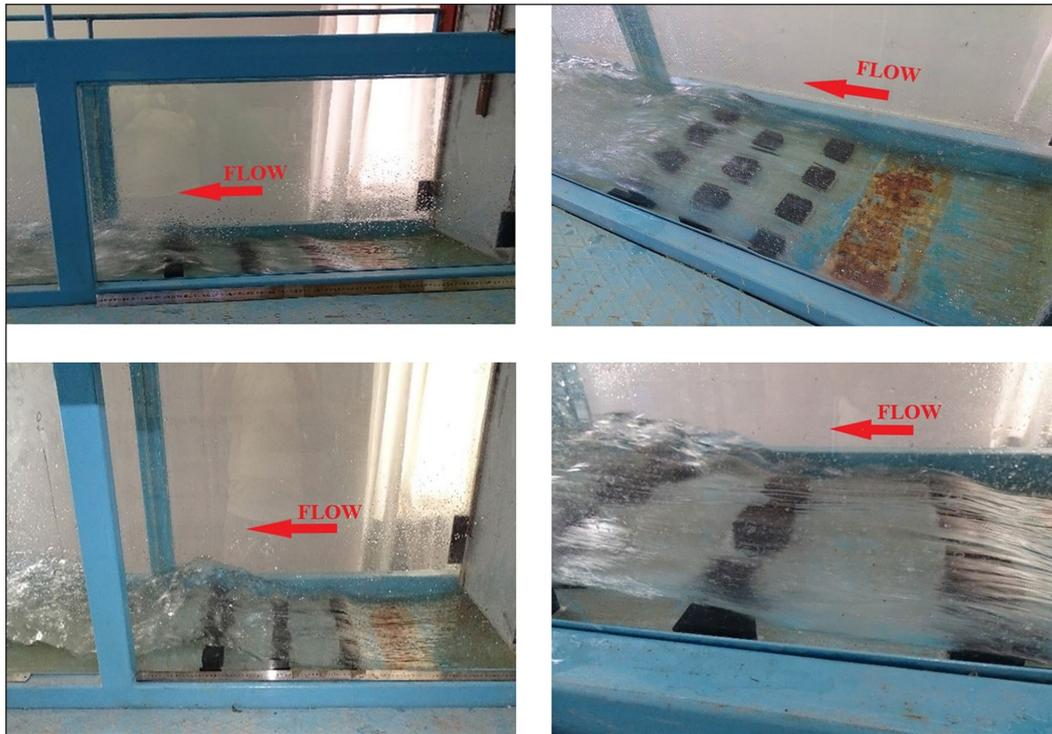
**Figure 3.** Experimental observations of hydraulic jumps due to the baffles downstream of the sluice gate
