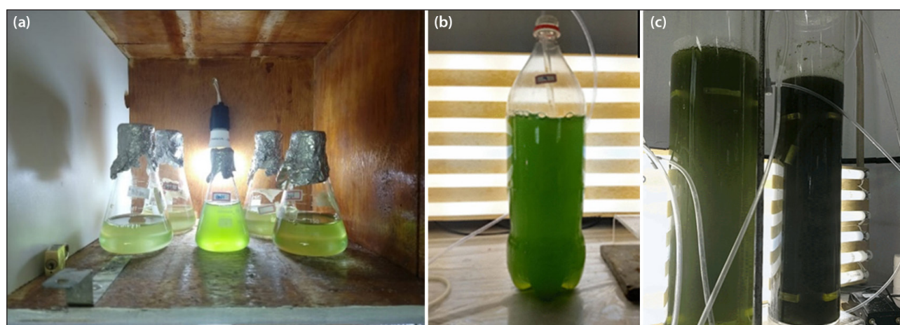
Figure 1. Stages of cultivation of Chlorella minutissima in landfill leachate: (a) Chlorella minutissima strain in the wood incubator, (b) transplant, and (c) airlift reactor cultivation stages
