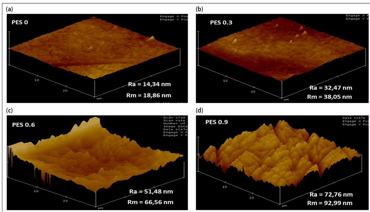
Figure 7. AFM images of (a) PES 0, (b) PES 0.3, (c) PES 0.6 and (d) PES 0.9 blended membranes evaluated at 2 x 2 μm scan area
