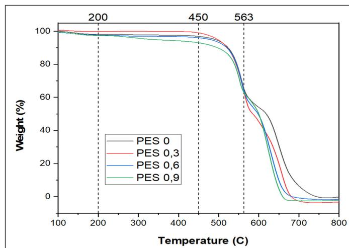
Figure 5. TGA analysis of PES and TA-Fe<sup>III</sup> complex of various loadings
