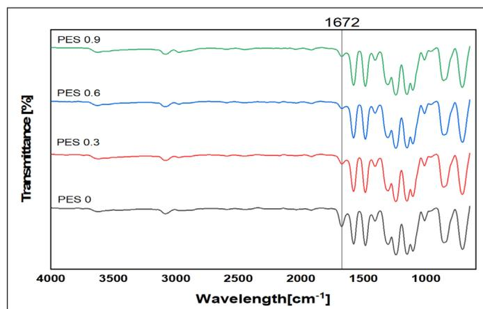
Figure 4. FTIR spectra of PES and PES blended membranes with various TA-Fe<sup>III</sup> complex loading
