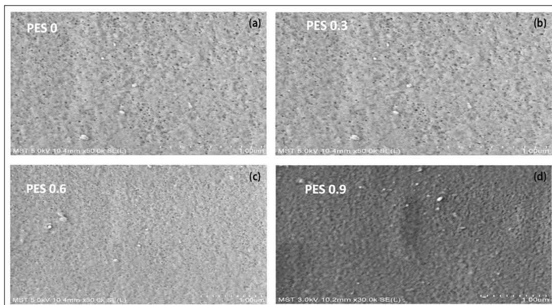
**Figure 1.** FE-SEM surface morphology of (a) PES 0, (b) PES 0.3, (c) PES 0.6 and (d) PES 0.9 blended membranes
