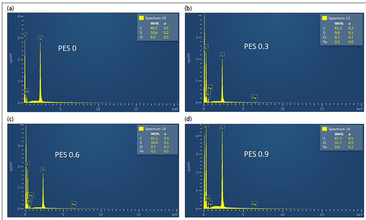
**Figure 2.** EDX results for different loadings of TA-Fe<sup>III</sup> complex in the fabricated PES membranes
