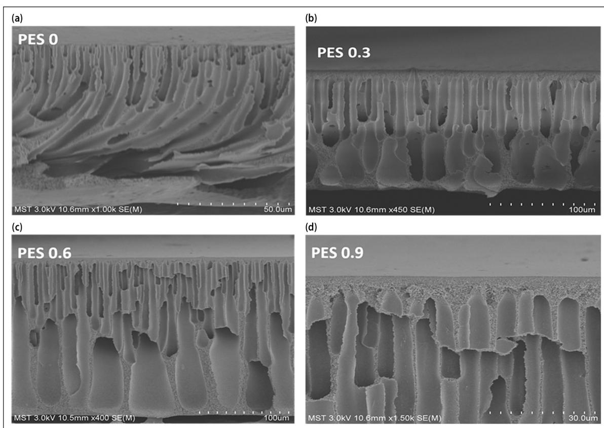
**Figure 3.** FE-SEM cross-sectional image of PES 0 to PES 0.9 blended membranes
