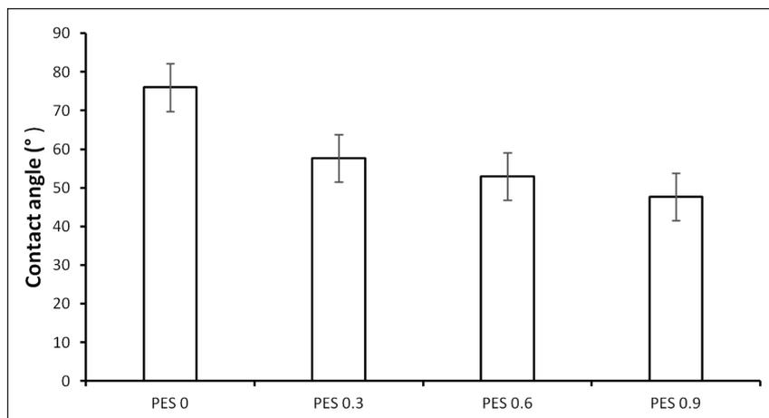
Figure 6. Contact angle of PES and PES modified with various TA-Fe<sup>III</sup> complex loadings
