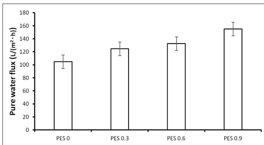
**Figure 8.** Effect of TA-Fe<sup>III</sup> complex loading on the pure water flux (PWF). Experimental conditions: temperature = 25°C, pressure = 100 kPa, time = 10 min
