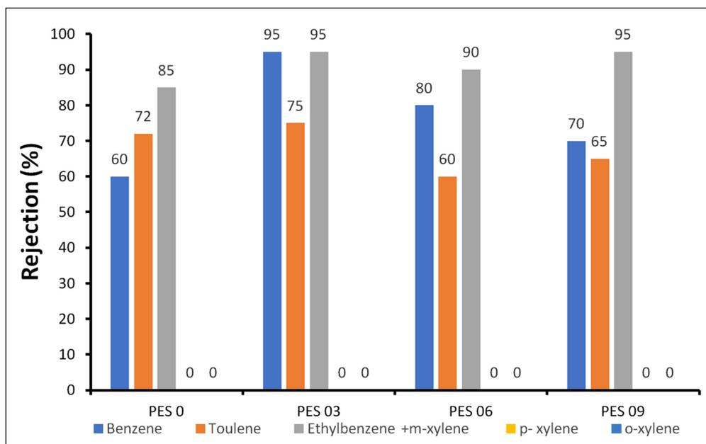
**Figure 9.** Rejection of benzene, toluene, ethylbenzene and xylenes using PES 0 and PES modified with various TA-Fe<sup>III</sup> complex loadings. Experimental conditions: temperature = 25°C, pressure = 100 kPa, time = 10 min
