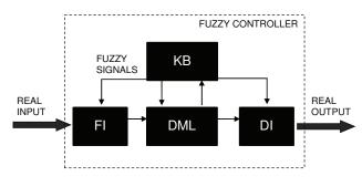
Figure 1 Fuzzy logic controller structure
