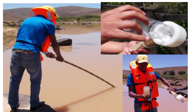
Figure 5 The wooden pole sampler in use showing the attachment of the sample jar into the head assembly.
